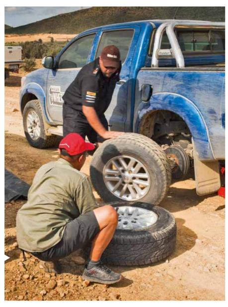
**Change, inflate, measure, fit... 64 times.** The tyre team operated like a well-oiled machine to ensure the completion of all 60 tests. Donovan Stanley of Klipbokkop (left front) and Brian Sadie from Tiger Wheel & Tyre (left) helped to fit all the rubber on our test Hilux.
